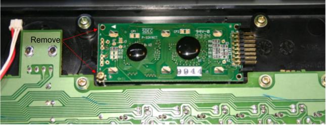
6) Place the new display over the top left locating peg and replace the screw from the previous step and attach the cable.
