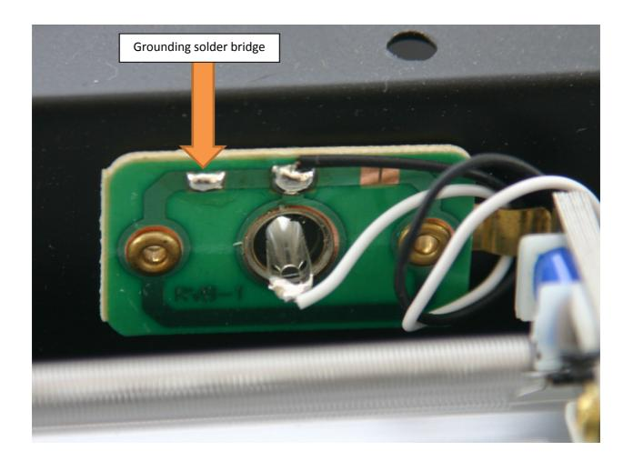
By way of example, we are going to convert an 8BB2A1B to an 8BB2C1B. Here is the bottom view of an 8BB2A1B. You can see that there are solder bridges on both connectors.
