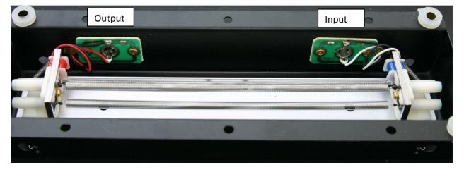
The 8BB2C1B has the input isolated so we need to remove the solder bridge by heating the solder until it is molten and quickly brush away the solder with a cotton bud or similar. A better choice, if you have it, is to use a product like 'solder wick' to remove the excess solder. Make sure no solder debris is left inside the chassis. That's it!
